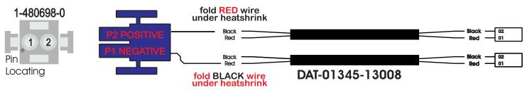
Mate-N-Loc Connector, Flat Face Down 2 Pin Part Number 1-480698-0 Tyco Pin Number 350570-1 Viewed with Tyco Connector Plug-In Face Down.
