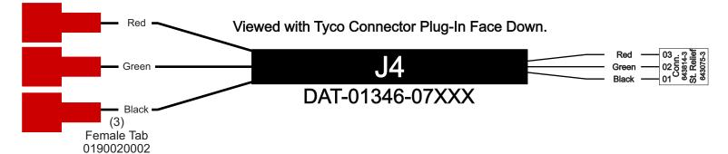
Carol C-4062, 22 AWG, Stranded, unshielded three conductor cable. Cut each jacket end 4 inches long, remove jacket on each end. Add heatshrink with DAT part number.
