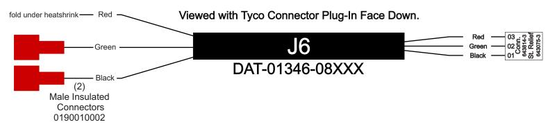
Carol C-4062, 22 AWG, Stranded, unshielded three conductor cable. Cut each jacket end 4 inches long, remove jacket on each end. Add heatshrink with DAT part number.
