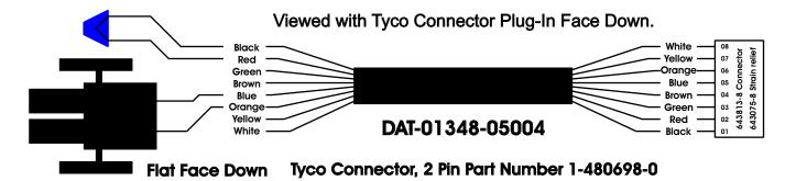
Carol C-2465, 22 AWG, Stranded 7/30/8, unshielded eight conductor cable. Cut each jacket end 4 inches long, remove jacket on each end. Requires one (1) Tyco/Amp. 643814-8 connector & Tyco/Amp. 643075-8 end cap. Place connector into insertion equipment, start with #8 and complete with #1
