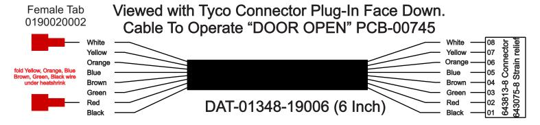
Carol C-2465, 22 AWG, Stranded 7/30/8, unshielded eight conductor cable. Cut each jacket end 4 inches long, remove jacket on each end. Add heatshirnk with DAT part number.
