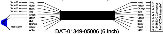
Operates Relays 4A, 4B, 5A and 5B with "IGNITION", on RCT-00786 or RCT-01414, Bus Power Center. Connects to J4-PCB-01083.
