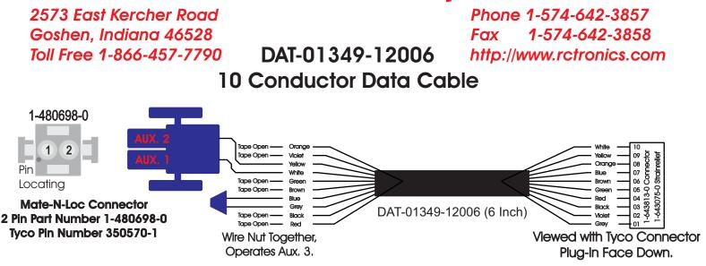
Mate-N-Loc operates relays Aux. 1 & Aux. 2 with "IGNITION", on RCT-01490 or RCT-01507, Bus Power Center connects to J4 on RCT-01544, Dash Switch Center.
