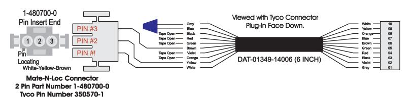
Mate-N-Loc operates relays Aux. #1 (Pin #1), Aux. #2 (Pin #2) and Heat (Pin #3) on Bus Power Center RCT-01507 with "IGNITION". Data Cable connects to PCB-01777-J3, Dash Switch Center.
