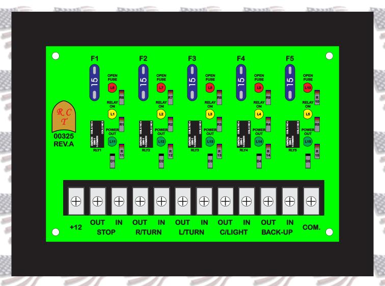
Five Relay with Relay On LEDs.
