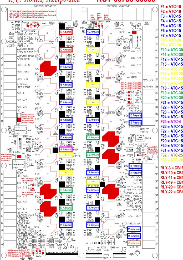
F1 = ATC-10F2 = ATC-10F3 = ATC-15 F4 = ATC-15F5 = ATC-15F6 = ATC-15F7 = ATC-15
