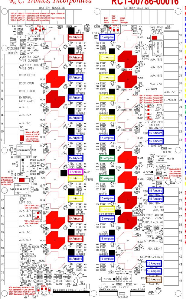
F1 = ATC-10F2 = ATC-10F3 = ATC-15 F4 = ATC-15F5 = ATC-15F6 = ATC-15F7 = ATC-15
