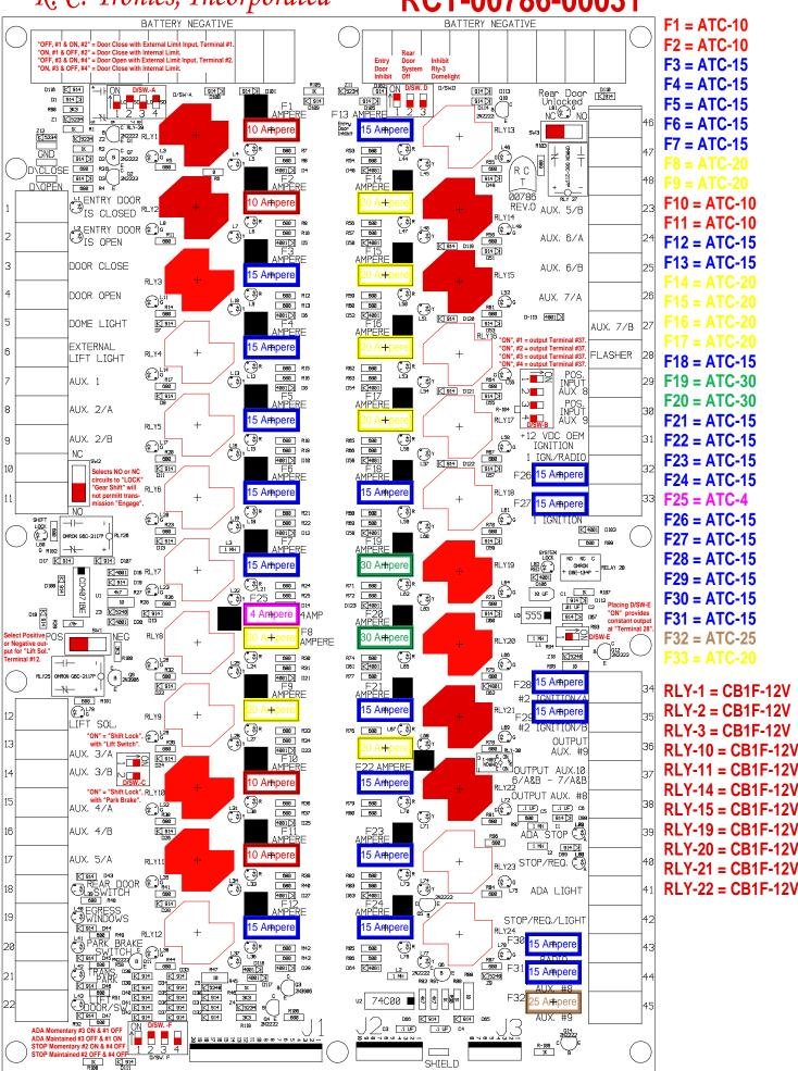
F1 = ATC-10F2 = ATC-10F3 = ATC-15 F4 = ATC-15F5 = ATC-15F6 = ATC-15F7 = ATC-15 F10 = ATC-10F11 = ATC-10F12 = ATC-15F13 = ATC-15F18 = ATC-15 F19 = ATC-30F20 = ATC-30F21 = ATC-15F22 = ATC-15F23 = ATC-15F24 = ATC-15F25 = ATC-4F26 = ATC-15F27 = ATC-15F28 = ATC-15F29 = ATC-15F30 = ATC-15F31 = ATC-15F32 = ATC-25RLY-1 = CB1F-12VRLY-2 = CB1F-12VRLY-3 = CB1F-12VRLY-10 = CB1F-12VRLY-11 = CB1F-12VRLY-14 = CB1F-12VRLY-15 = CB1F-12VRLY-19 = CB1F-12VRLY-20 = CB1F-12V
