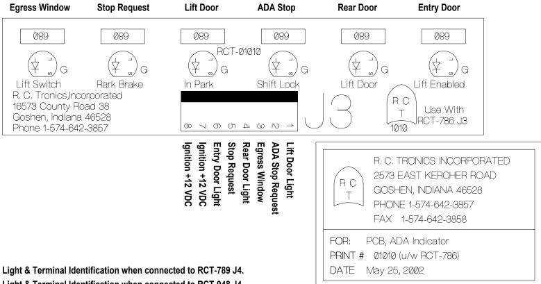
Light & Terminal Identification when connected to RCT-948 J4.
