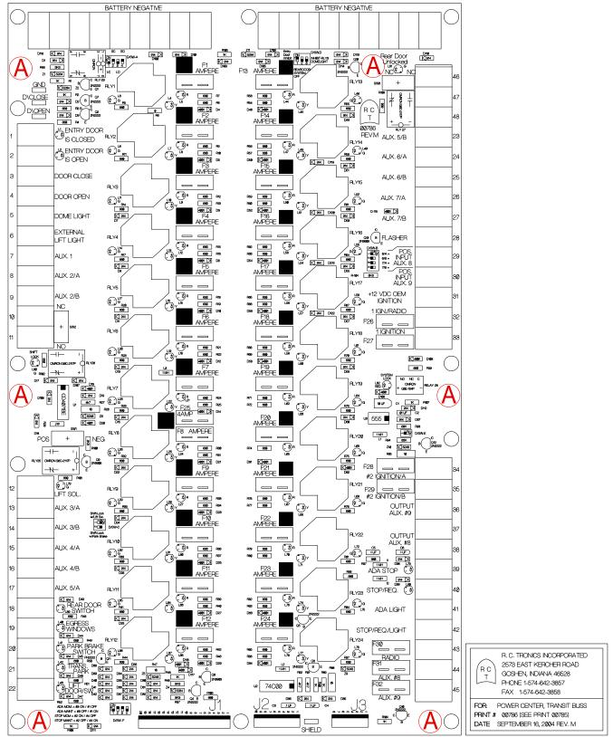
Note #1 Six Mounting Openings, .5 Inch. Do Not Capture PCB with Screw Head PCB May Crack Causing Malfunction Use # 8 or # 10 Screw & Center In Opening.
