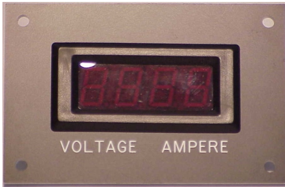
RCT-394 Alternates Voltage & Amperage
